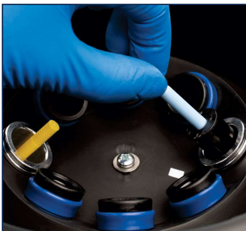
Insert the carrier in the metal tube sleeves.
